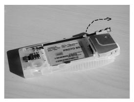
Antenna: Apply pressure with a nonconductive tool to snap the antenna out from the D-cover.
