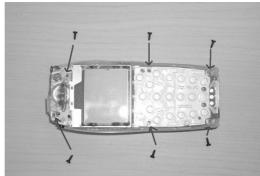
Remove the six screws using a nonconductive screwdriver.
